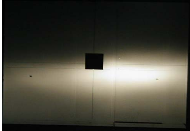
Figure 16. A TYC Taurus low beam pattern aimed with the vertical VHAD.
