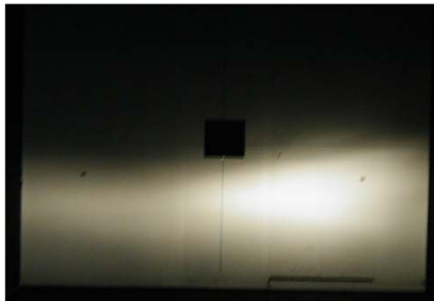
Figure 15. A Taurus original equipment manufacturer (OEM) replacement low beam pattern aimed with the vertical VHAD.
