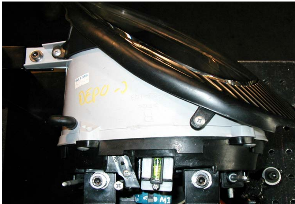
Figure 9. Top view of a DEPO manufactured Taurus headlamp. The bubble level (located near the bottom center) is a vertical VHAD used for setting the vertical aim.
