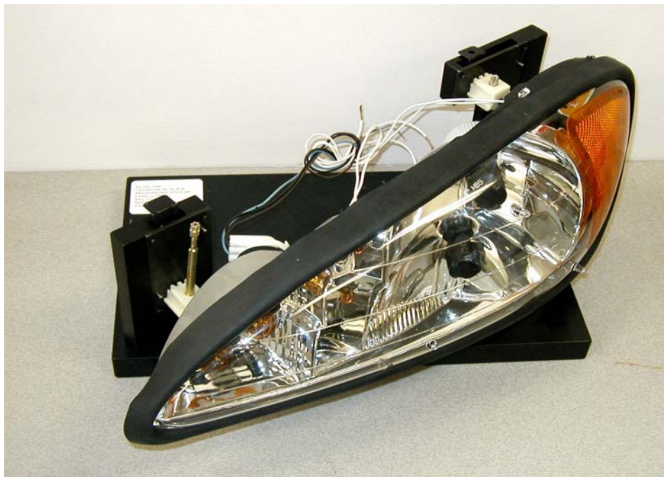
Figure 4. 1999-2003 LH Grand Am headlamp mounted on the photometric test fixture.
