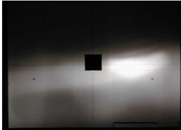
Figure 13. A TYC Grand Am low beam when aimed using the lens exterior aiming pads.
