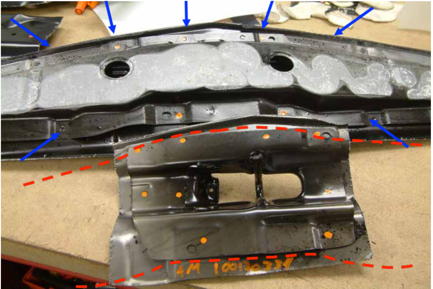
Figure 2: Missing Striker Reinforcement Plate
