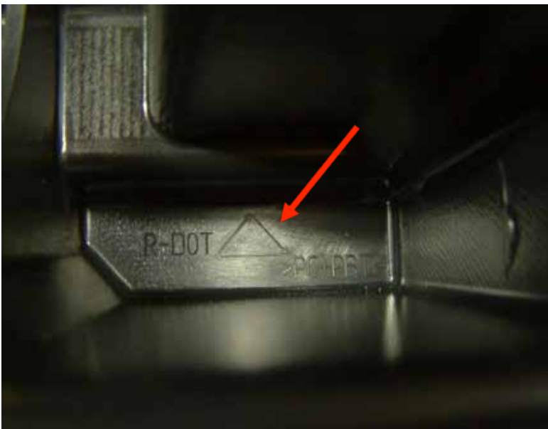
Figure 6: Fraudulent Material Marking on Non-CAPA Certified Aftermarket Part
