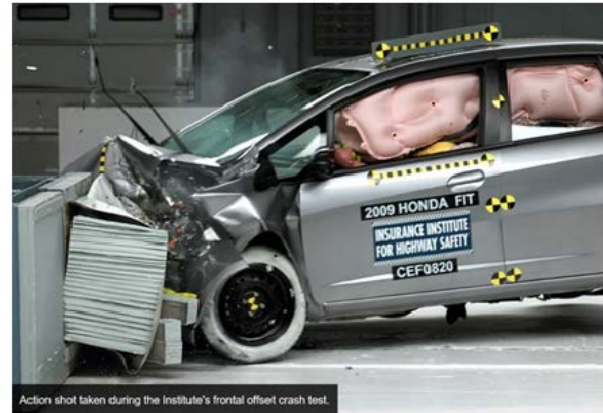
Action shot taken during the Institute's frontal offset crash test.
