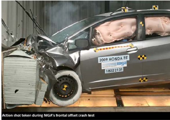
Action shot taken during MGA's frontal offset crash test
