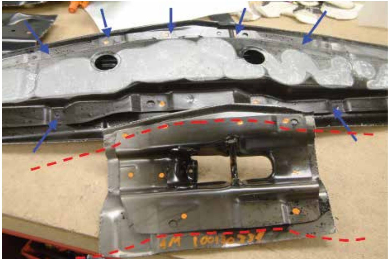
Figure 1: Missing Striker Reinforcement Plate
