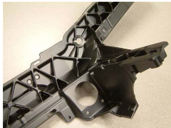
Figure 5. Close-up of BMW brand upper tie bar for the Convertible. Both the cast aluminum material and honeycomb structure stiffen the part and give it very different strength properties from the radiator support manufactured by BMW for its Sedan/Coupe/Wagon.
