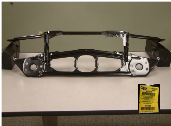
Figure 3. CAPA Certified Gordon radiator support replacing BMW part #51717111691 for 1999-2006 BMW 3-Series Sedan/Coupe/Wagon (as received). This part cannot be used on the convertible.
