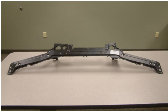
Figure 1. BMW-made radiator support #51717114123 – Upper Tie Bar for 1999-2006 BMW 3-Series Convertible (as received).
