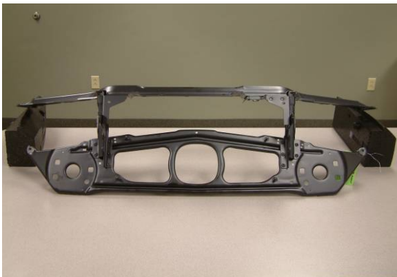
Figure 2. BMW-made radiator support #51717111691 for 1999-2006 BMW 3-Series Sedan/Coupe/Wagon (as received).
