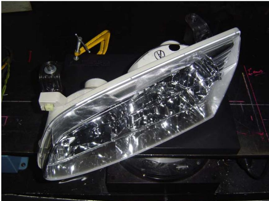
**Figure 10. 2000-2001 LH Toyota Camry headlamp mounted to the goniometer table.**
