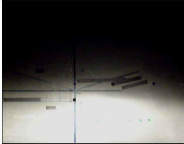
**Figure 11.** A Ford Taurus original equipment manufacturer (OEM) replacement low beam when aimed using the VOR method.
