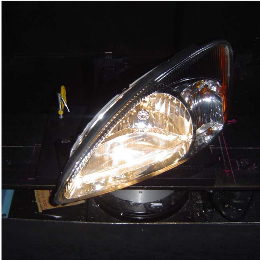
**Figure 9. 2000-2003 LH Ford Taurus headlamp mounted to the goniometer table.**
