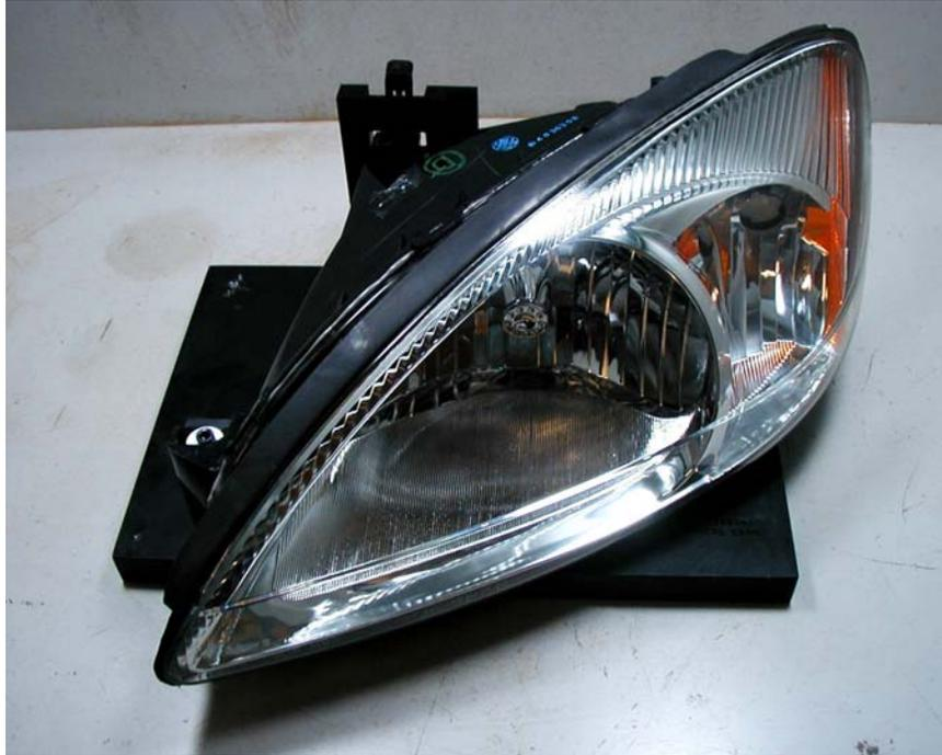
**Figure 5. 2000-2003 LH Ford Taurus headlamp mounted on the photometric test fixture.**
