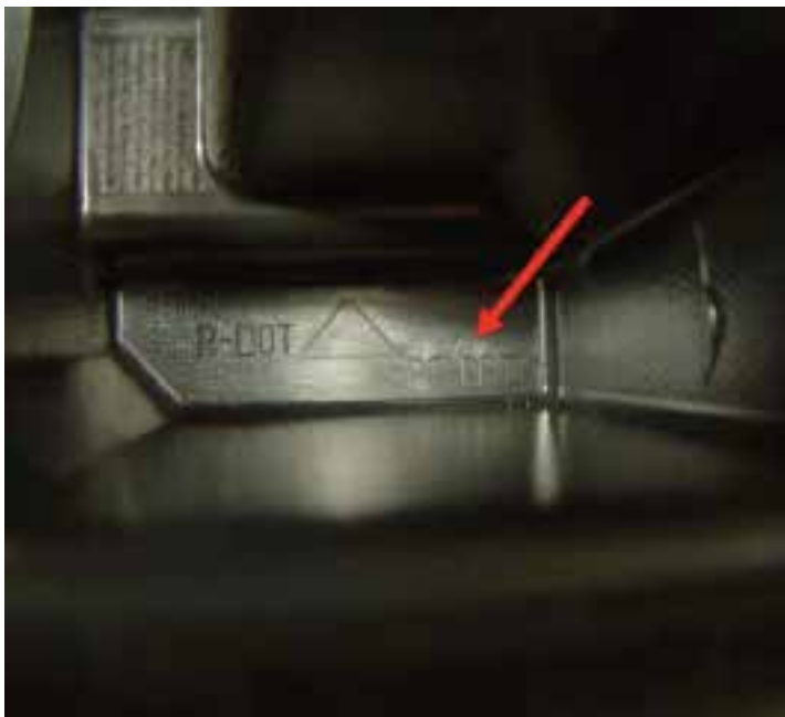
Figure 3: Fraudulent Material Marking on Non-CAPA Certified Aftermarket Part
